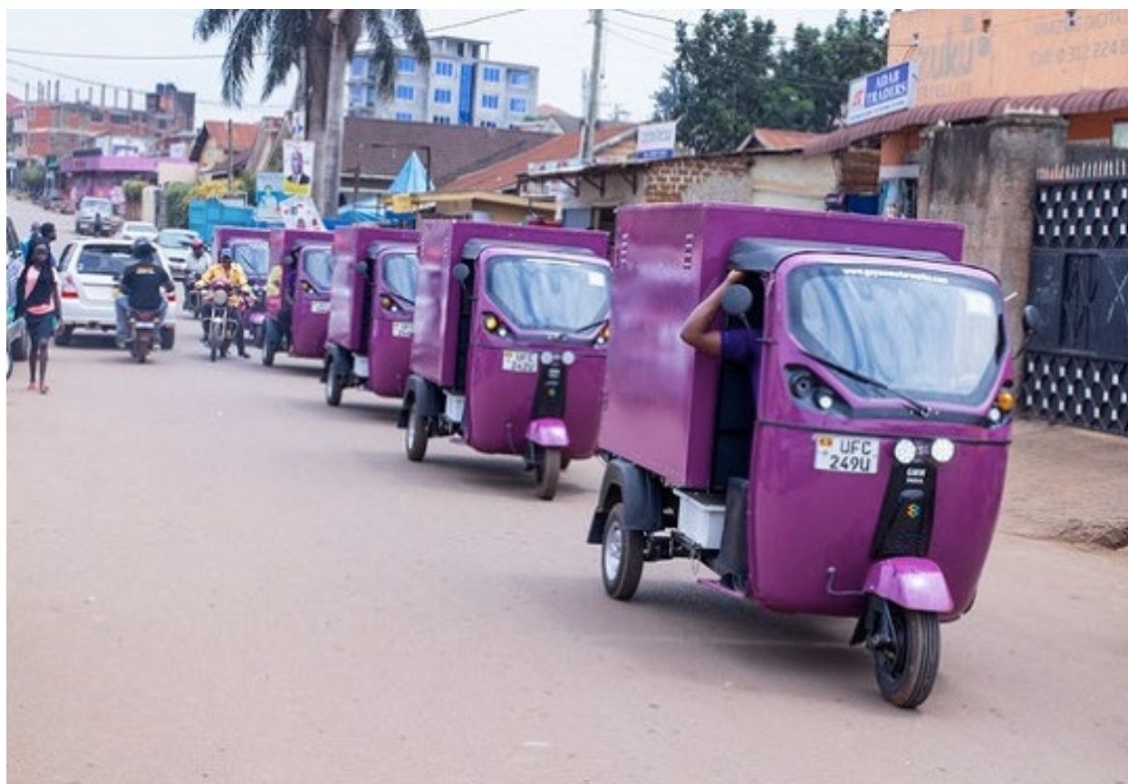
Image 1: Sokowatch, the innovative East African e-commerce platform, has launched electric three wheelers, commonly referred to as tuk-tuks, to its delivery fleet in Uganda, making the vehicles the first to be used commercially in East Africa. The new fleet of vehicles take 3 hours to charge and last for approximately 2-3 days, and can carry 500kg in goods.
